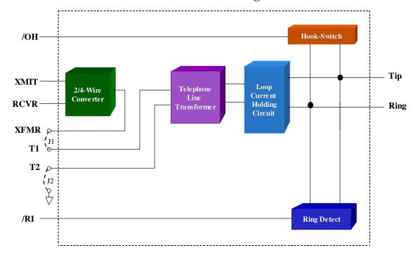
Jumpers J1 and J2 must be installed to connect the 2 to 4 wire convertor.
